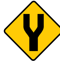
Yellow diamond 'Y' sign (road divides ahead)
