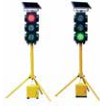
Mobile traffic signal device (temporary traffic lights sometimes used on roadwork. The same rules apply for these as normal traffic lights)
