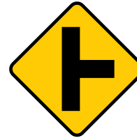
Yellow diamond side-on 'T' sign (a side road meets the road you are travelling on)
